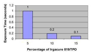
Figure 4. Cure speed versus phosphine oxide photoinitiator content.
