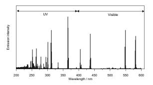
Figure 2. Typical Medium Pressure Mercury Emission Spectrum
