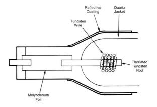
Figure 1. Schematic of a medium pressure mercury arc lamp electrode
